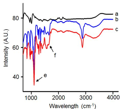
**Fig 3.** FT-IR characterization (a: IONPs; b: IONP-loaded polymer nanoassemblies; c: IONP/DOX co-entrapped polymer nanoassemblies; e: ether peak at 1,100 cm<sup>-1</sup>; and f: amide peak at 1,650 cm<sup>-1</sup>).
