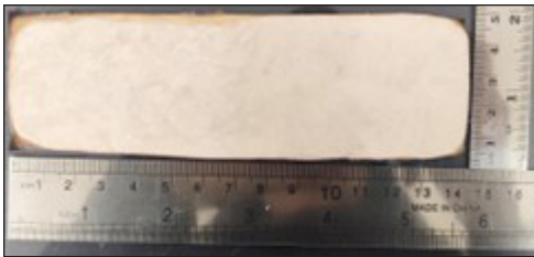
Figure 4. Dry BC film after casting onto glass plates.
