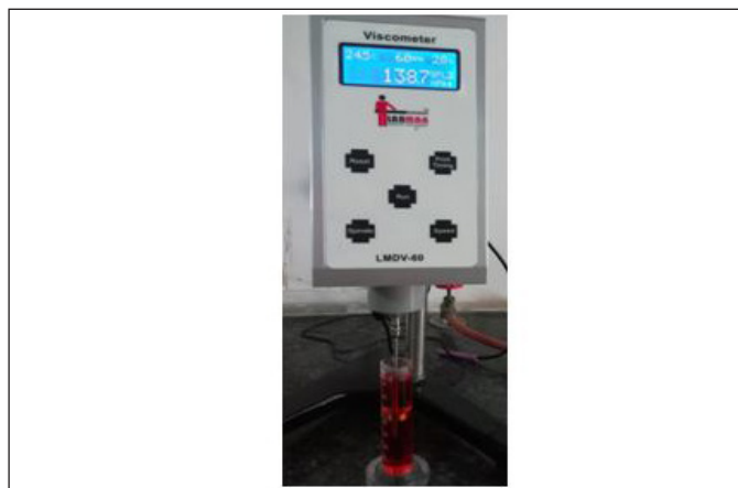
Figure 14. Measurement of viscosity of saffron nanoemulsion under digital viscometer.
