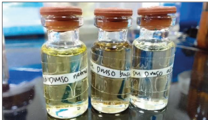
Figure 3. Color change of the chromophore on 1-(2,5-dihydroxyphenyl)-3-pyridine-2-yl-propenone under DMSO solvent conditions, from left to right: neutral, alkaline, acidic.
