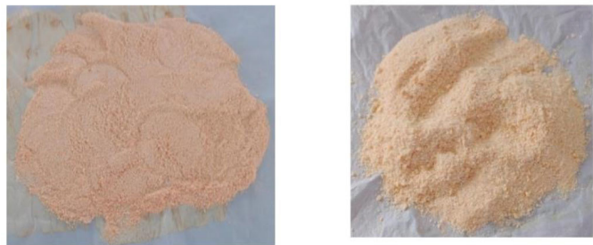
Figure 1. The results of chitin isolated from waste and chitosan from lobster shells.
