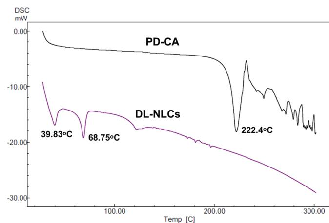
Figure 2. DSC thermogram of pure drug (CA) and DL-NLCs.
