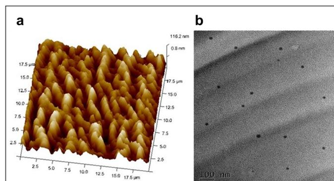
Figure 3. AFM (a) and TEM (b) images of CA loaded NLCs.
