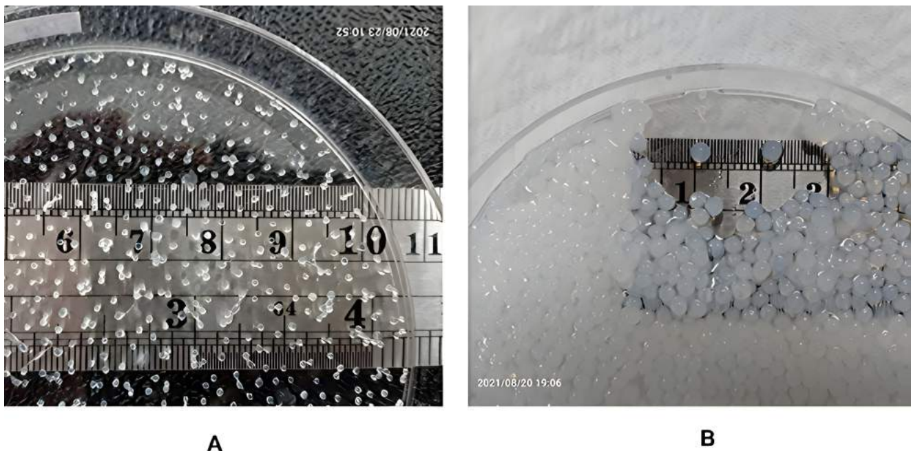
Figure 5. Swelling of CS-PEGDA beads. (A) Dried beads before soaking and (B) swollen beads after soaking in PBS buffer pH 7.4 for 24 hours.
