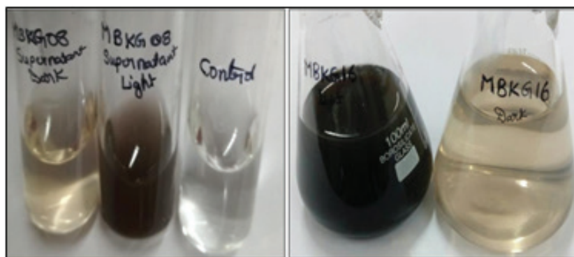
Figure 1. Synthesis of silver nanoparticles under light and dark conditions.
