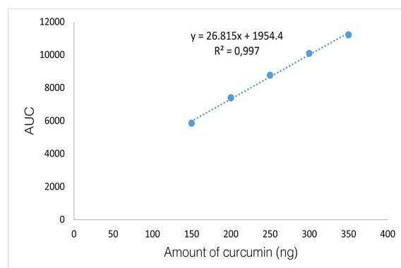
Fig. 2: Calibration curve of curcumin.
