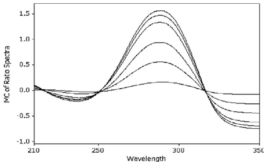
**Fig. 6:** Mean centering of ratio spectra for different concentrations (2.00 -24.00  $\mu\text{g/mL}$ ) of CFD at 288.4 nm using acid degradation products (40.00  $\mu\text{g/mL}$ ) as divisor.
