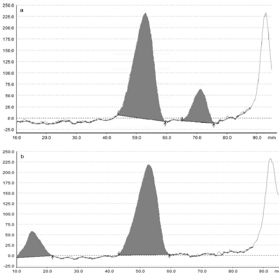
**Fig. 8:** HPTLC chromatograms of mixture solutions containing CFD 2.00 µg/spot with its acid (a) and alkaline-(b) degradation products (1.00 µg/spot each).
