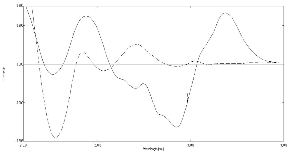
**Fig. 3:** Second derivative (<sup>2</sup>D) absorption spectra of CFD (—) and its acid degradation products (- -) (24.00 µg/mL each).
