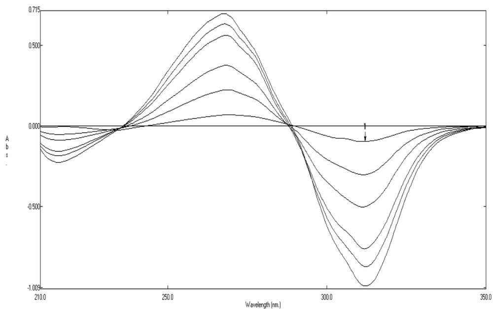
**Fig. 4:** First derivative of ratio spectra (<sup>1</sup>DD) for different concentrations (2.00 -30.00 µg/mL) of CFD at 312 nm using acid degradation products (40.00 µg/mL) as divisor.
