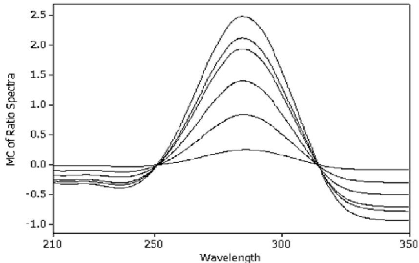
**Fig. 7:** Mean centering of ratio spectra for different concentrations (2.00 -26.00  $\mu\text{g/mL}$ ) of CFD at 284.8 nm using alkaline degradation products (40.00  $\mu\text{g/mL}$ ) as divisor.
