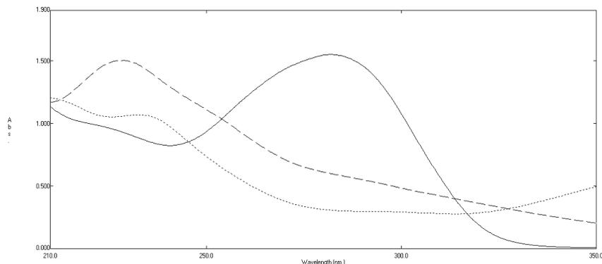
**Fig. 1:** Zero order absorption spectra of CFD (—), its acid (- -) and alkaline degradation products (...) (24.00 µg/mL each).
