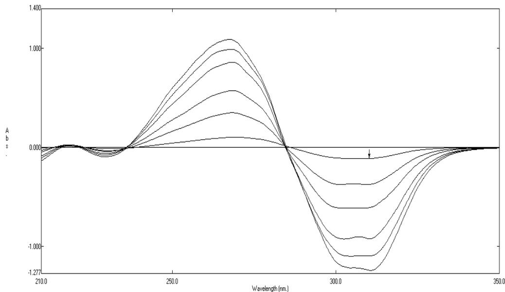
**Fig. 5:** First derivative of ratio spectra ( $^1DD$ ) for different concentrations (2.00 -30.00  $\mu\text{g/mL}$ ) of CFD at 310.2 nm using alkaline degradation products (40.00  $\mu\text{g/mL}$ ) as divisor.
