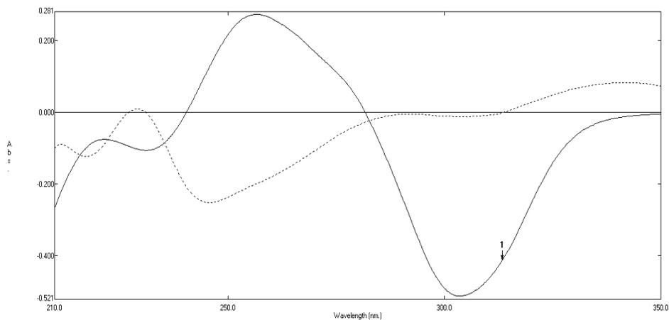
**Fig. 2:** First derivative (<sup>1</sup>D) absorption spectra of CFD (—) and its alkaline degradation products (...) (24.00 µg/mL each).
