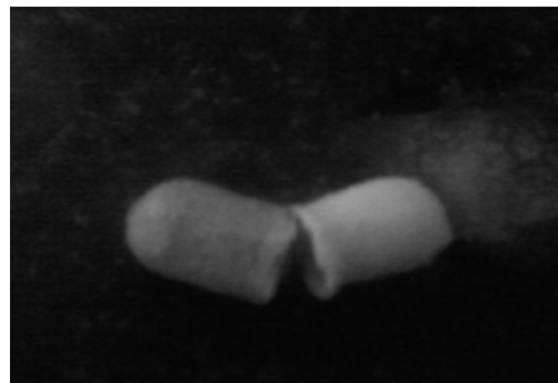
Fig. 7: Capsule disintegration and drug dissolution at pH 6.8 PBS (Capsule of 89 \mu m thicknesses).
