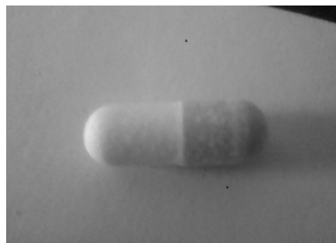
Fig. 3: Enteric coated capsule after 2h in 0.1N HCl.
